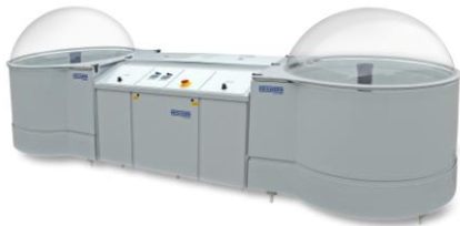
Model 606-2 with 2 test chambers 1000 l circular
