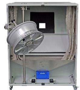
In the Impact Cabinet **RIMpact I VDA**, the wheel rim to be tested is turnably fixed, so **each single spoke** can be tested differently by choice with varying combinations of shot gravel, shoot cycles, shot gravel quantities, shoot periods and shoot pressures (**under an impact angle of 90°**).
