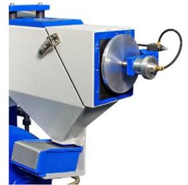
Attachment for tests in accordance with Daimler DBL 5416, for vertical impact angle at 90°, with infinitely adjustable shoot distance.
