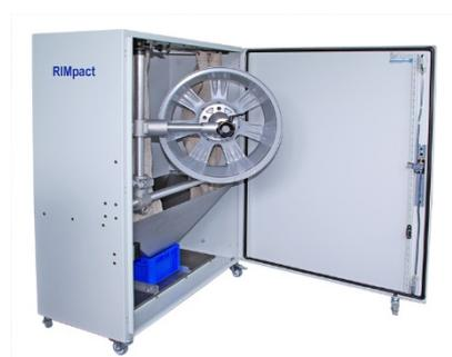
Enables the user to test complete rims respectively in principle also several other specimen, which up to now – due to their big sizes – would have to be previously segmented by cutting them.
