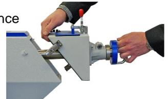
Impact cabinet **RIMpact II VDA** for stone impact simulation testing at rims/wheels up to 26" dia. x 335 mm width (**under consideration of 54° impact angle prescribed by VDA, in connection with the correct shoot distance**). The variable holding device allows an upright positioning as well as to tilt the sample's position.
