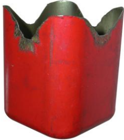
Square Deep Drawing Cup Test
