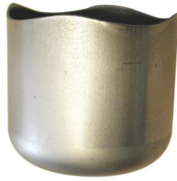
Deep Drawing Cup Test
