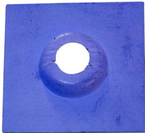
Bore Expanding Test
