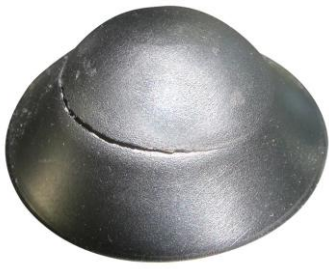
ERICHSEN Cupping Test
